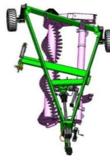
Shipping kit installed ready for truck
